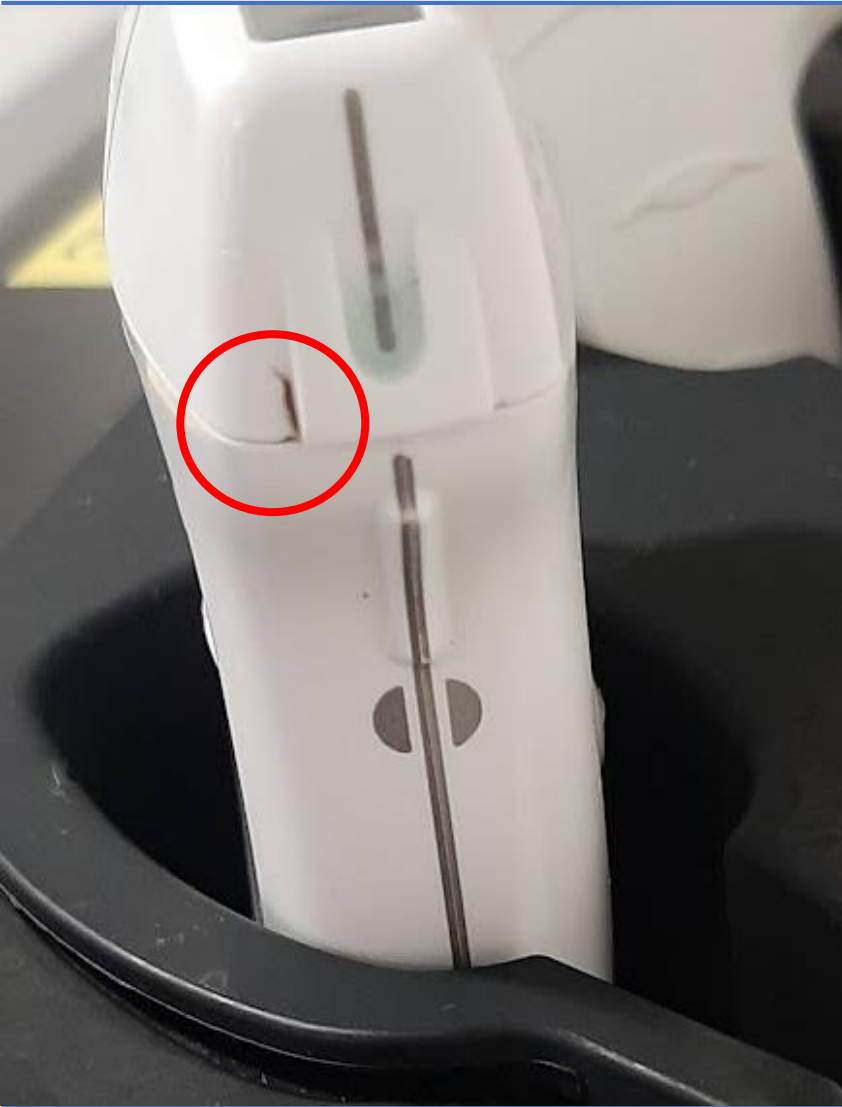
Blood And Gel Remain On Probe For Next Operator To Use
