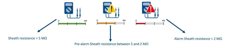
Automatically controls the integrity of your probe according to EN 60601-1 as required manufactures
